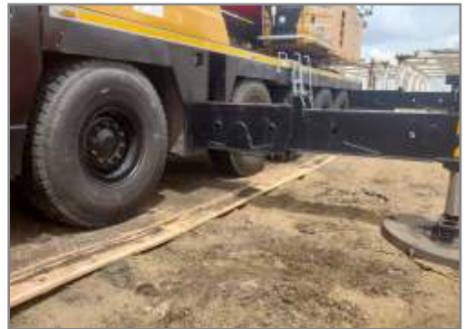
Area Each Mat: 4m x 2m Thickness: 94mm Material Strength: 425Ton/Sq.m Weight (Per Sheet): 360Kg.
