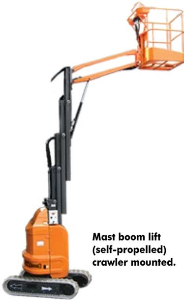
**Mast boom lift (self-propelled) crawler mounted.**
